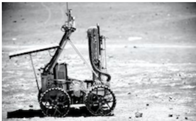
Heavily studded wheels are a key design feature.
