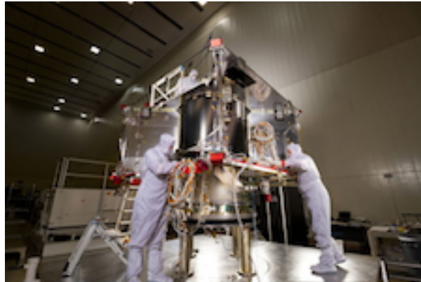
Lockheed Martin technicians in a clean room facility near Denver assembled NASA's OSIRIS-Rex asteroid-sampling spacecraft
