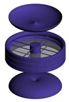
Figure 10 - Expanded Vademecum with micro-gravity center, twin mirrors and solar panels
