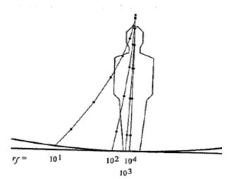
Figure 19: Dropped a ball in artificial gravity: relationship of floor radius to trajectory deflection
