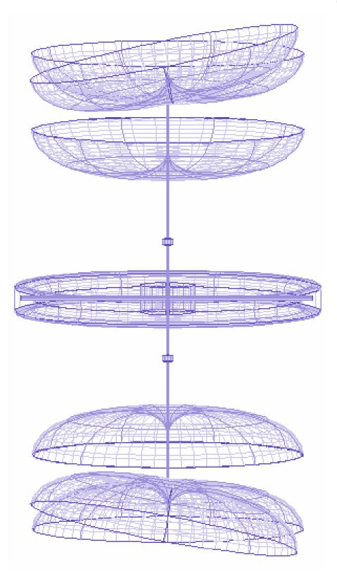
Figure 16 - Vademecum with flexible mirrors (moving up/down and tilting sideways to maximize exposure to sunshine)
