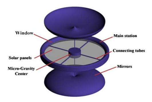
Figure 8 - Vademecum with micro-gravity center, twin mirrors and solar panels - Side view
