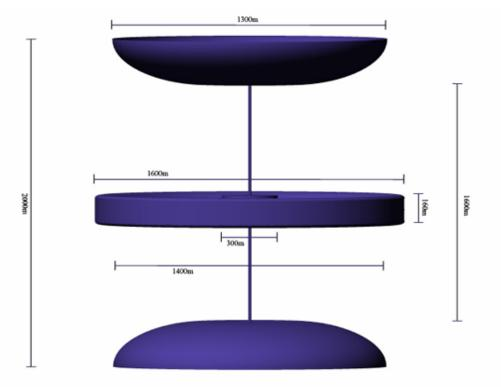
Figure 9 - Vademecum with micro-gravity center, twin mirrors- Cross Section
