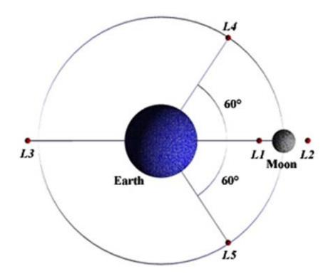
Figure 12 - The five Lagrangian points in a two-body system (e.g., the Earth and the Moon)
