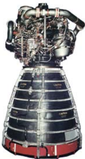
Figure 6-84. RS-25 (Altitude-Start SSME)
