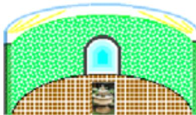
**Illustration** of a simple and small “greenhub” node, an intersection of 3 or 4 pedestrian passageways. It sports a higher vaulted ceiling, painted a matte sky blue, with cove uplit with bright sunshine spectrum bulbs. Vertical surfaces are living walls. The floor is of brick pavers or cobblestones, with a scattering of benches, flowerpots, and a central fountain. Connecting pedestrian walkways are lower in vertical scale.
