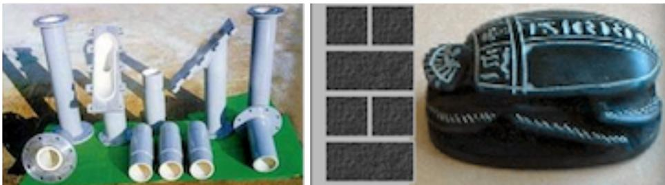
**L: Cast Basalt Pipes R: Hewn & Carved Basalt**
