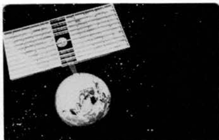
D11 Power satellite of the photovoltaic type (Arthur D. Little).
